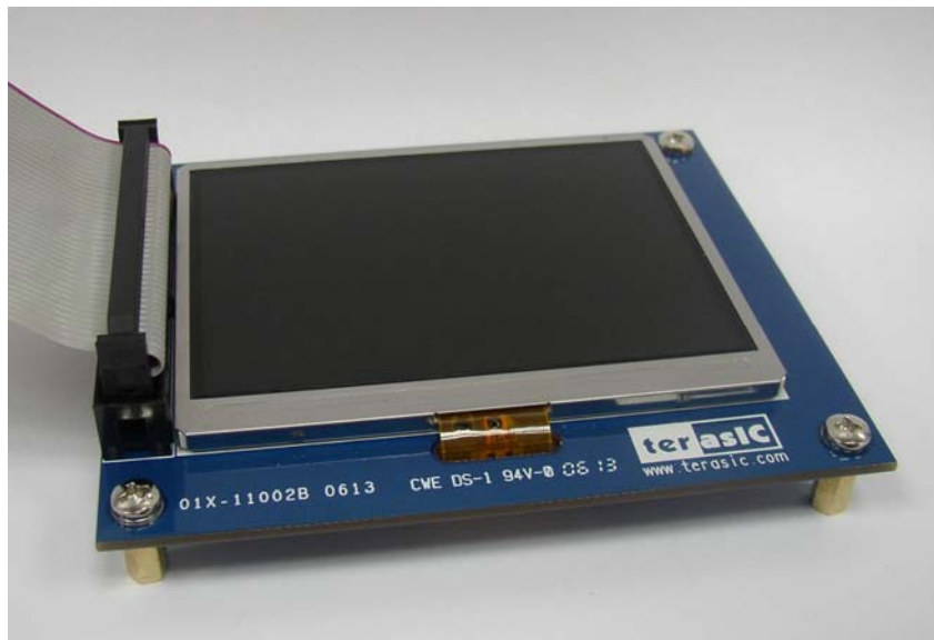
Figure 1.2 Connect the IDE cable to the TRDB_LCM board
